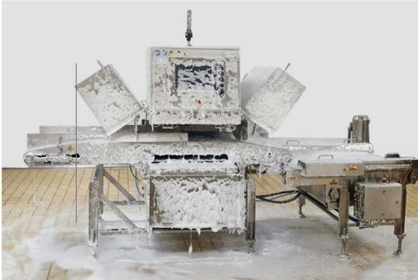
Figure 9: Equipment must be capable of withstanding rigorous, high-pressure, high-temperature wash down procedures.
