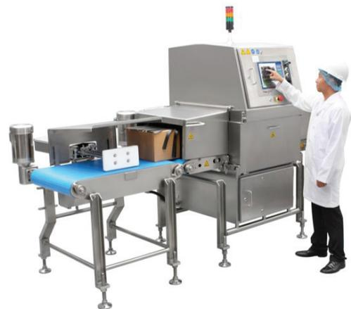
Figure 7: Buttons on control panels should be easily cleanable so as not to create a microbial harborage.
