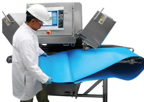
Figure 2: Contact surface materials should be corrosion resistant, non-toxic and non-absorbent.
