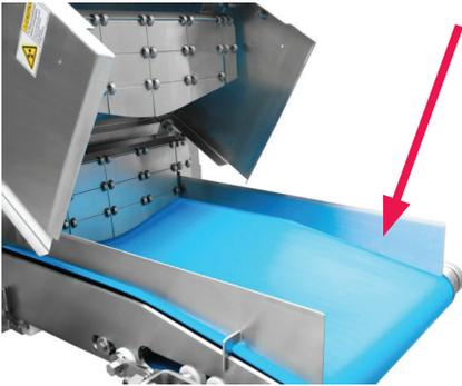
Figure 8: Example of sloped belt construction.
