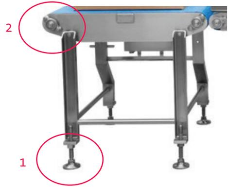
Figure 5: (1) No hollow areas in frames and rollers. (2) No Hollow areas at or above the product contact zone.
