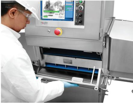
Figure 3: Equipment designed to increase accessibility for cleaning is vital and reduces downtime by making cleaning easier and quicker.
