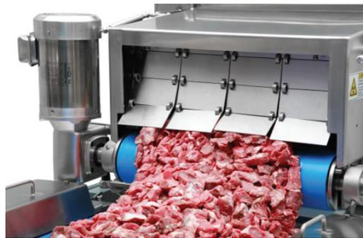
Figure 1: Smooth, regular surfaces help to prevent microorganism growth.
