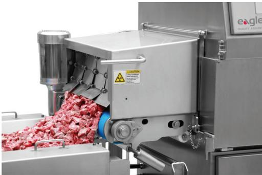
Figure 4: Framework should be rounded or inclined at 45 degrees, and flat under surfaces that are difficult to see or clean should be avoided.
