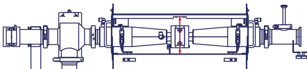
Eagle™ Pipe Manifold Inspection Area, front open cabinet view, provides a uniform area to maximize detection capabilities at 2.5", 3", 4" and 6" pipe diameters.
