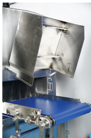
Figure 5: Hinged louvers allow easy access to the conveyor
